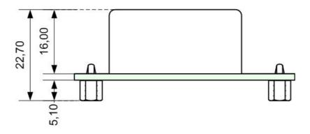
The default mounted feet can be easily removed.
